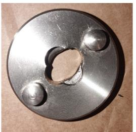
Non-conforming suspension: The BPPA axis and BPPA shoulder cannot be removed from the suspension.
